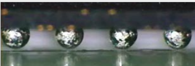
Real-time rework process visualization of BGA during reflow
