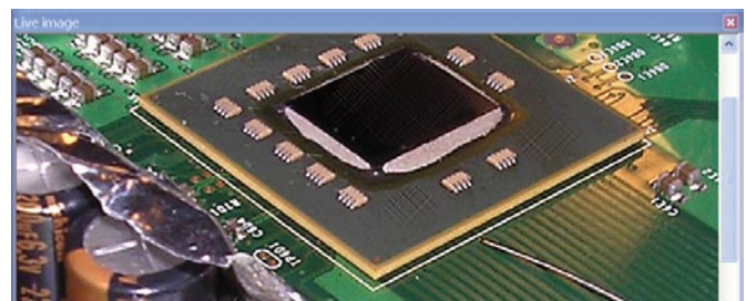
Rework process visualization with Live Image Window
