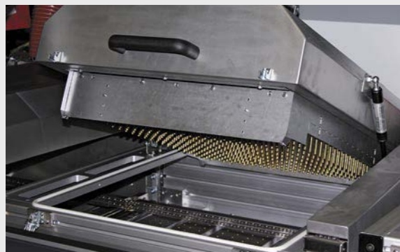
Top & Bottom Side Convection Heating Modules
