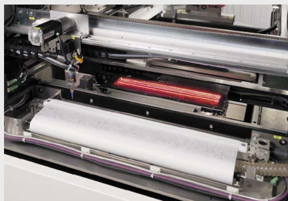
Intelligent Stencil Cleaner via 100 % Inspection
