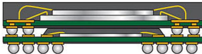
Juki machines are ideally suited for PoP (Package on Package) applications. PoP is a placement method which allows a higher vertical placement density and makes a component construction kit possible. Memory components can, for example, be placed freely onto logic modules creating a more cost effective solution that allows memory size to be freely adapted to the market needs.
