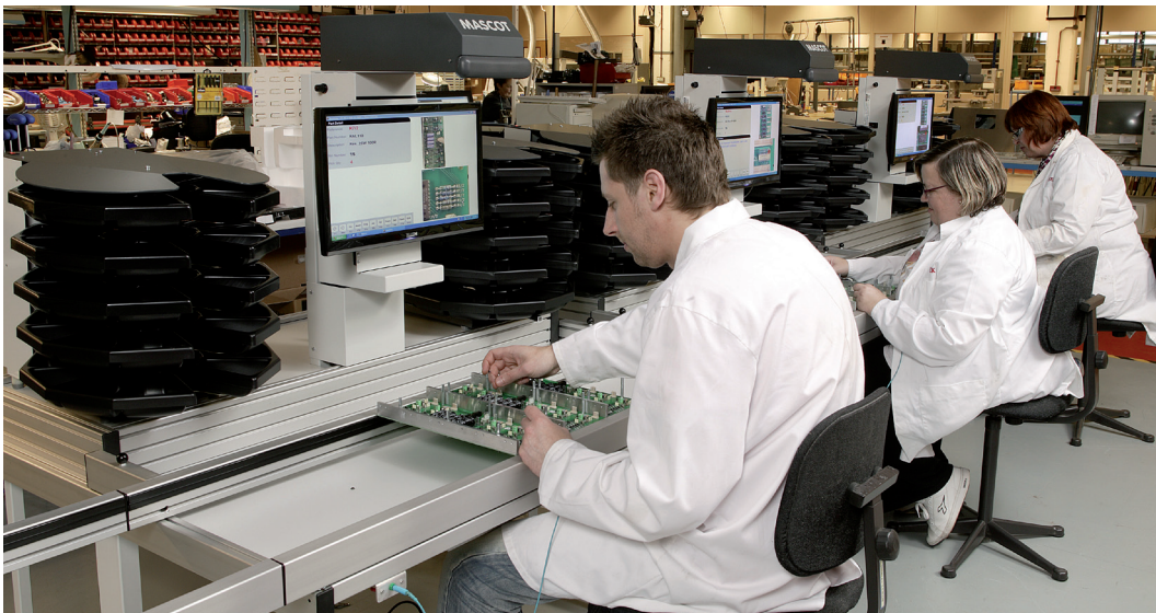
MASCOT Pushtracks working in a 'Lean Line' configuration
