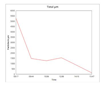
Placed in a canteen of  $40m^2$  for a period of eight hours. Particle readings were taken over that period of time. Results shown are of the total number of microns in  $\mu m$  as shown by the particle reader.
